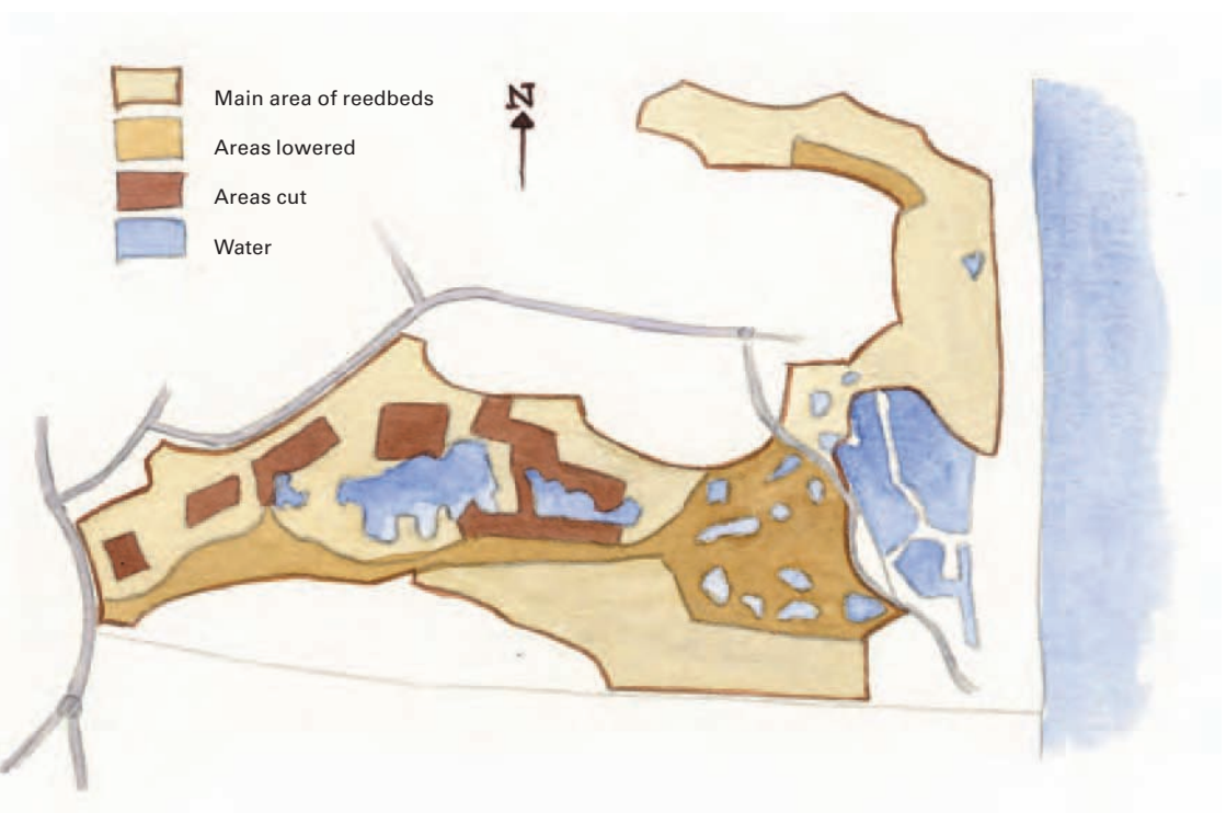
Figure 7.6 The Minsmere Reserve showing the extent of the main reedbeds, the zones subject to periodic cutting and the areas lowered between 1991 and 2000.
