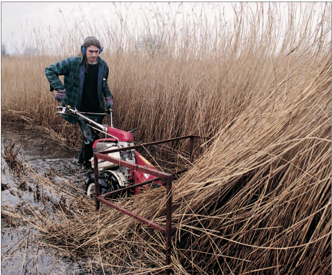
Plate 5.3 Cutting and gathering reed using a reciprocating mower.
