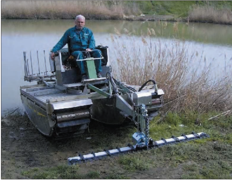
Plate 5.7 The Aquaclear 'Truxor'; a versatile amphibious reedcutter.
